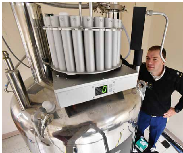
Lt. Col. Dan Harrison '05 inspects the Auto Sample Changer, an addition to the nuclear magnetic resonance spectrometer, in Maury-Brooke Hall.—VMI Photo by Kelly Nye.
