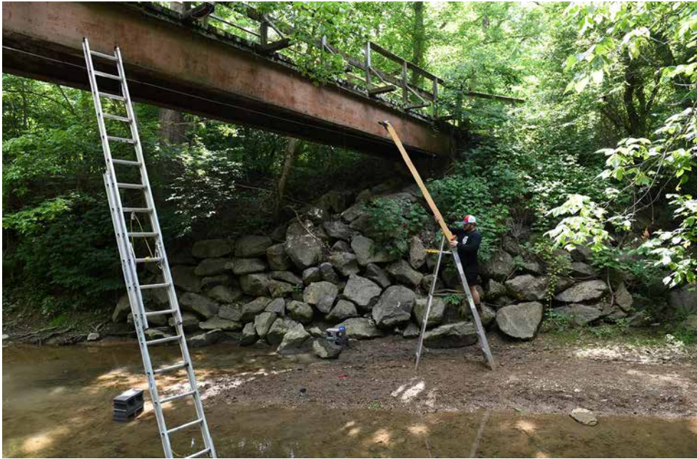
Lawrence Porter '24 sets up equipment to run tests on the serviceability of a footbridge on the Chessie Nature Trail.—VMI Photo by Marianne Hause.
