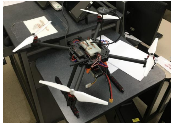
Figure 2: Completed X4 Drone Assembly
