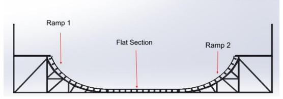
Figure 1. Final CAD Model outlining the three major sections
