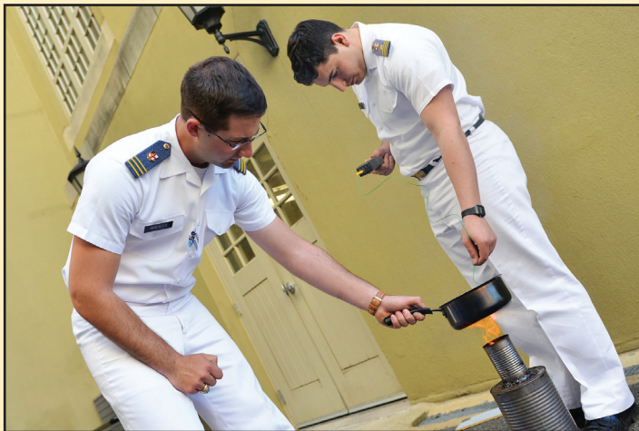
Tyler Brickles '15 and Peter Buehlmann '15 check the temperature of a pan of water heated over a cooking stove designed to refine llama droppings for use in biochar water filters. – VMI Photo by John Robertson IV.
