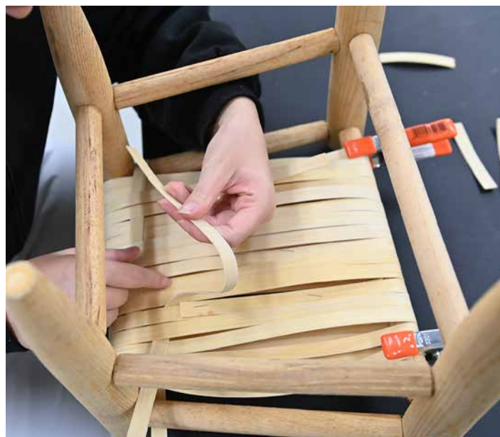
Flat reed strips are woven to make the seat of a chair.—VMI Photo by Kelly Nye.
